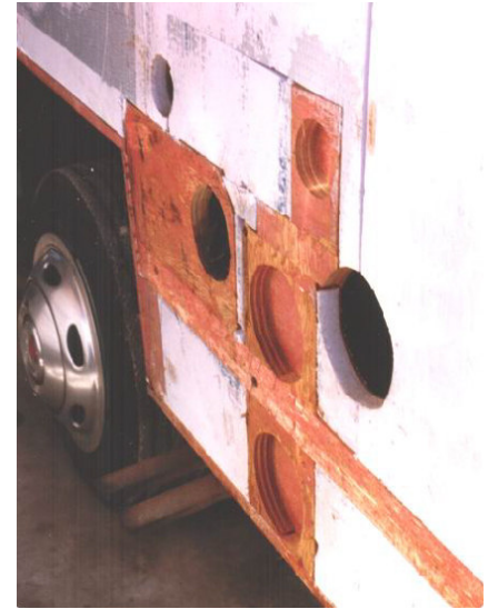
Laminate separation discovery. Notice the six holes. Mistakes covered up by the manufacturer. This is common.
